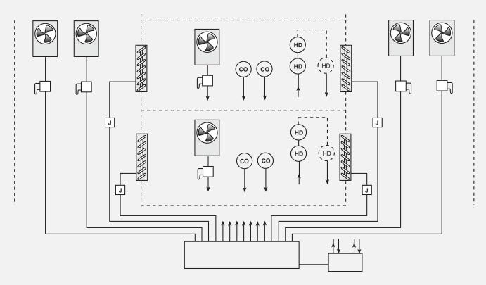
Colt can provide a full system comprising control panels, carbon monoxide (CO) detection, and an addressable heat/smoke detection system. Alternatively our control panels can be linked to the building's fire alarm system..
